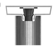
Insert the cradle into the HDTK: Aluminum Display Track with the t-nut inside the track as shown.
