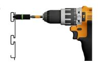
Place screw guide into channel at stud location. Firmly press both guide and drill against rail and drive screw through channel into stud.
