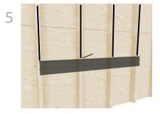
If stacking multiple rails: Extend lines vertically to the full height of the display and recheck stud alignment. Transfer stud marks to channel.
