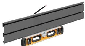
Hold rail against wall with the stacking tab down as shown above. Check level and draw a line along the top of the rail.
