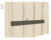
Extend lines vertically to the full height of the 30" display and recheck stud alignment.
