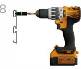
Place screw guide into channel at stud location. Firmly press both guide and drill against rail and drive screw through channel into stud.
