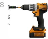
Place screw guide into channel at stud location. Firmly press both guide and drill against rail and drive screw through rail into channel.
