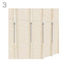
Mark lines vertically to the full height of the display and recheck stud alignment.
