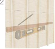
Hold rail against wall, check level and draw a line along the top of the rail. Using your preferred method, locate and mark every stud along the line.
