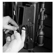
1. Run cable loop through trigger guards
