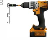
Place screw guide into channel at stud location. Firmly press both guide and drill towards rail and drive screw through channel into stud.
