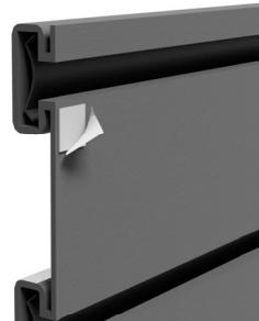
Remove paper backing from white adhesive square. Place face down on rail as shown. Remove paper backing from second side and align end cap for desired finish
