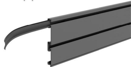
Insert screw cover strip from end of rail if accessible, otherwise press into slot with pen or marker.
