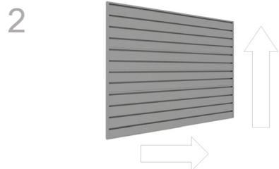
Choose a location and height for your 4'W X 3'H display taking into consideration clearance required to add and remove firearms from racks. Begin installation with the lowest row of rails.
