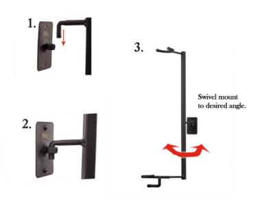
Choose location for mount. Drive screws through mounting holes of mount into wall using a phillips screwdriver. We recommend mounting this stand directly into wall studs.
