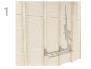
Locate studs, double check 16" on centers. Assure height of rack allows room to remove your longest barreled rifle.
