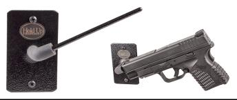
Choose location for hanger. Drive screws through mounting holes of hanger into wall using a Phillips screwdriver. If a wall stud is not found, these pilot holes are necessary for installing the drywall anchors. To do this, use the screwdriver to push and turn the anchor clockwise until flush. Remount hanger with screw into anchor. DO NOT REUSE ANCHORS.
