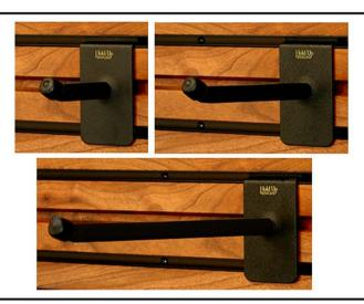
Choose location for hanger. Drive screws through mounting holes of hanger into wall using a Phillips screwdriver. If a wall stud is not found, these pilot holes are necessary for installing the drywall anchors. To do this, use the screwdriver to push and turn the anchors clockwise until flush. Remount hanger with screw into anchor. DO NOT REUSE ANCHORS.
