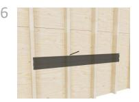
Using your preferred method, locate and mark every stud along the line. NOTE: Studs must be within 7" of the end of the rail. When joining rails end to end, if a stud aligns with joint of the two rails, move display 1" left or right.
