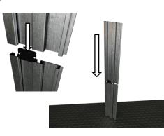
Press rails together. Grasping the top rail, tap rails on a rug or a non-marring surface to close gap.
