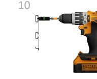
Place screw guide into channel at stud location. Firmly press both guide and drill against rail and drive screw through channel into stud.
