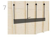
Mark lines vertically to the full height of the display and recheck stud alignment.
