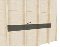
Using your preferred method, locate and mark every stud along the line. NOTE: Studs must be within 7" of the end of the rail. When joining rails end to end if a stud aligns with joint of the two rails, move display 1" left or right.
