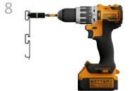
Place screw guide into channel at stud location. Firmly press both guide and drill towards rail and drive screw through channel into stud.
