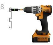
Place screw guide into channel at stud location. Firmly press both guide and drill towards rail and drive screw through channel into stud.
