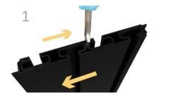
Rails will be nested back-to-back for safe shipping. Be sure to separate before assembling. (It may be necessary to use a screwdriver to separate rails)
