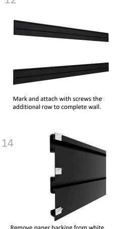
Remove paper backing from white adhesive square. Place face down on rail as shown. Remove paper backing from second side and align end cap for desired finish.
