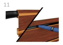
Insert black strip from end of rail if accessible, otherwise press into slot with pen or marker
